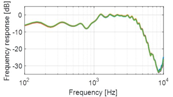
*Frequency response measured of an IP30 in a 711 coupler using the Sanibel™ insert foam tip*
